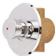
PRESTO 55 PULSADOR CAUDAL: 15 l/m REGULABLE CIERRE AUTOMATICO 30 s +5-10 1/2" H-H
