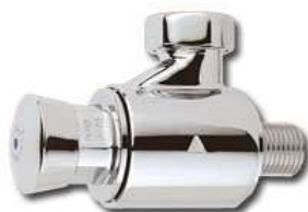
PRESTO 75 PULSADOR CAUDAL: 10 l/m REGULABLE CIERRE AUTOMATICO 30 s +5-10 1/2" M
